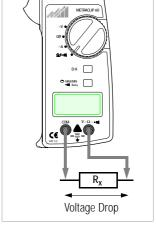
selector switch to the  $\mbox{\rm OFF}$  position. Restore the measuring circuit to its original condition.
